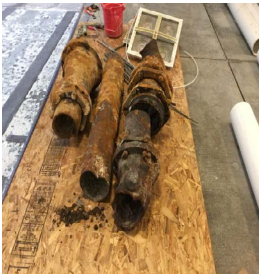
(old drain removed and new pipe installed)
