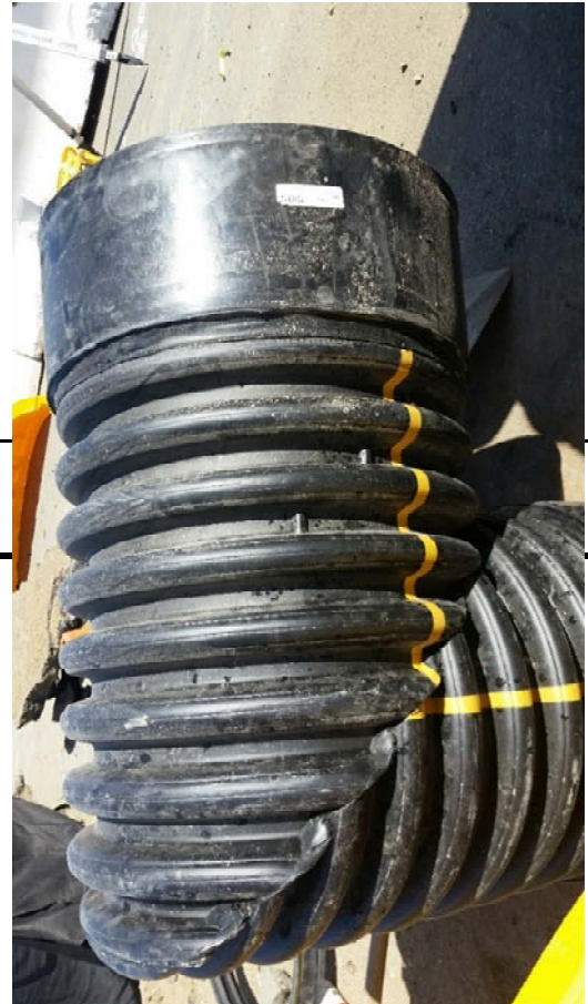
Infiltrator manhole end
