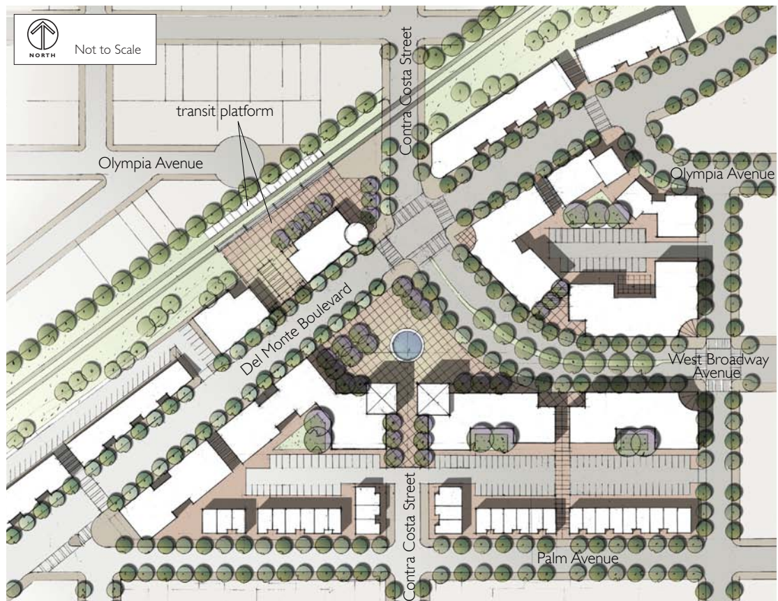
Figure 3-2. Realigned Intersection of West Broadway Avenue and Del Monte Boulevard (for illustrative purposes only)
