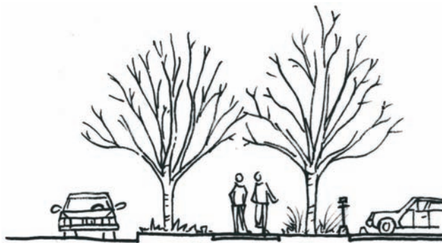
Parking buffered by landscaping.
