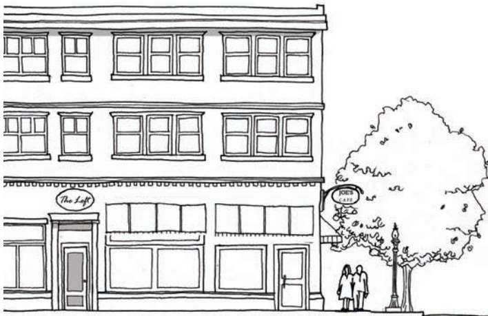
Recessed entry to upper level floor uses.
